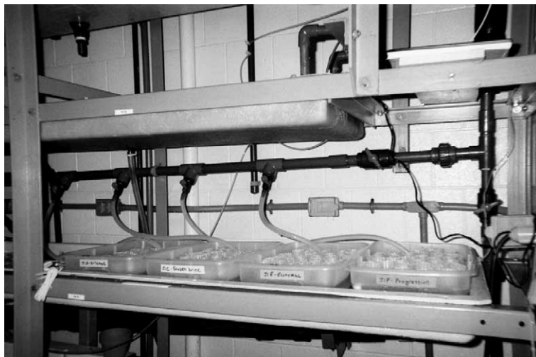
Fig. 1. The experimental setup for experiments One and Two. All rearing cups for a single diet are placed within a flow-through tub in a flow-through seatray. Water depth was approximately 5 cm.
